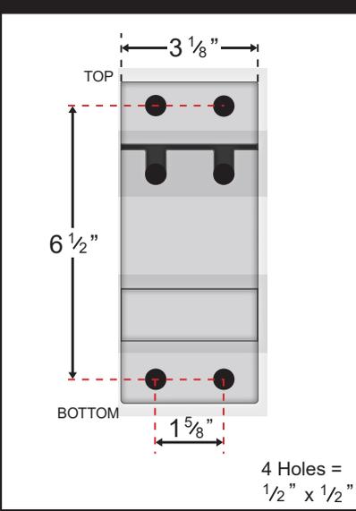
Wall and Soffit Bracket - Side View
